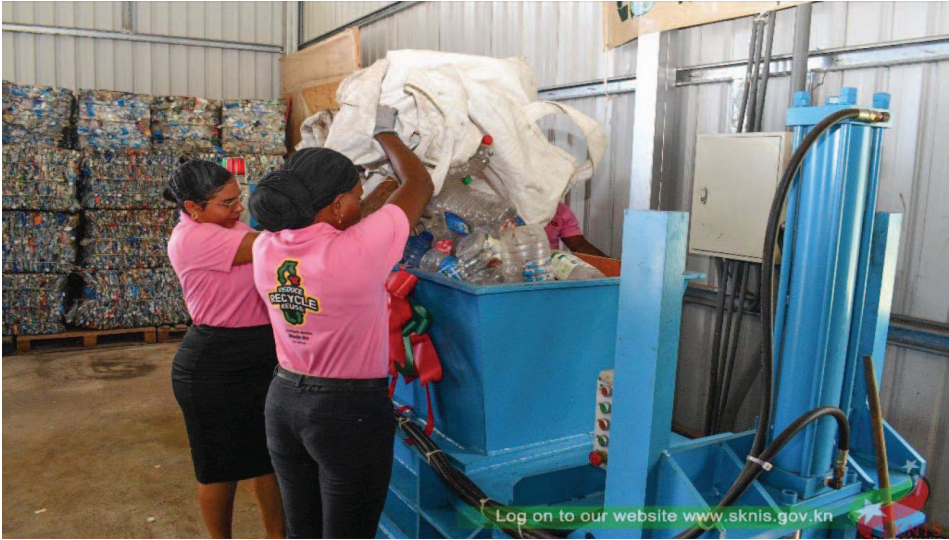
SWMC workers demonstrate how the baler works, loading plastic bottles
