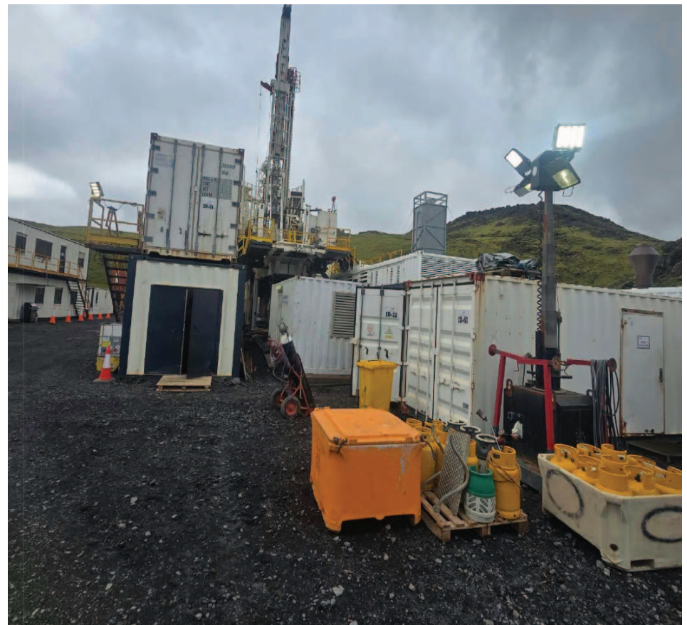
Drilmec HH-300 “Týr” rig undergoing final inspection at the Iceland Drilling Company facility ahead of mobilization to Nevis
