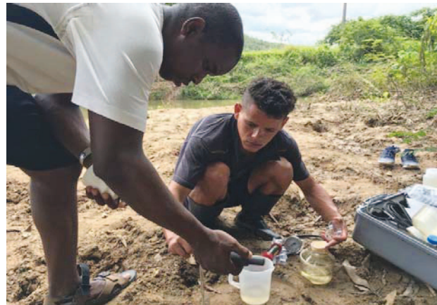
Cuban scientists Aniel Arruebarena and Victor Perez filter sediment from river water in western Cuba so that elements dissolved in the water can be analyzed accurately. Photo credit: Paul Bierman (CC BY-ND).
